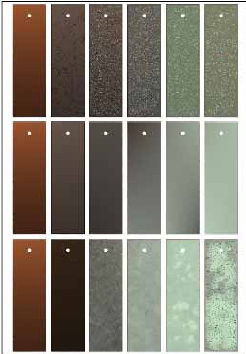
Figure 8: Copper time lines: marine environment (top); rural environment (middle); urban environment (bottom).
